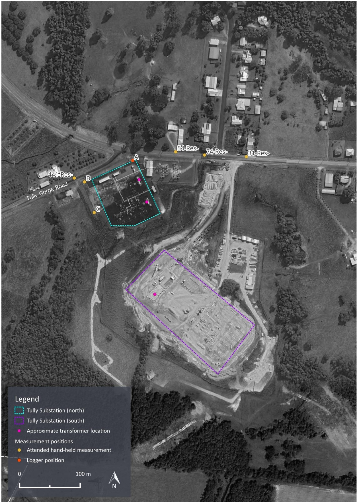
Figure 5: Tully substation noise survey location plan
