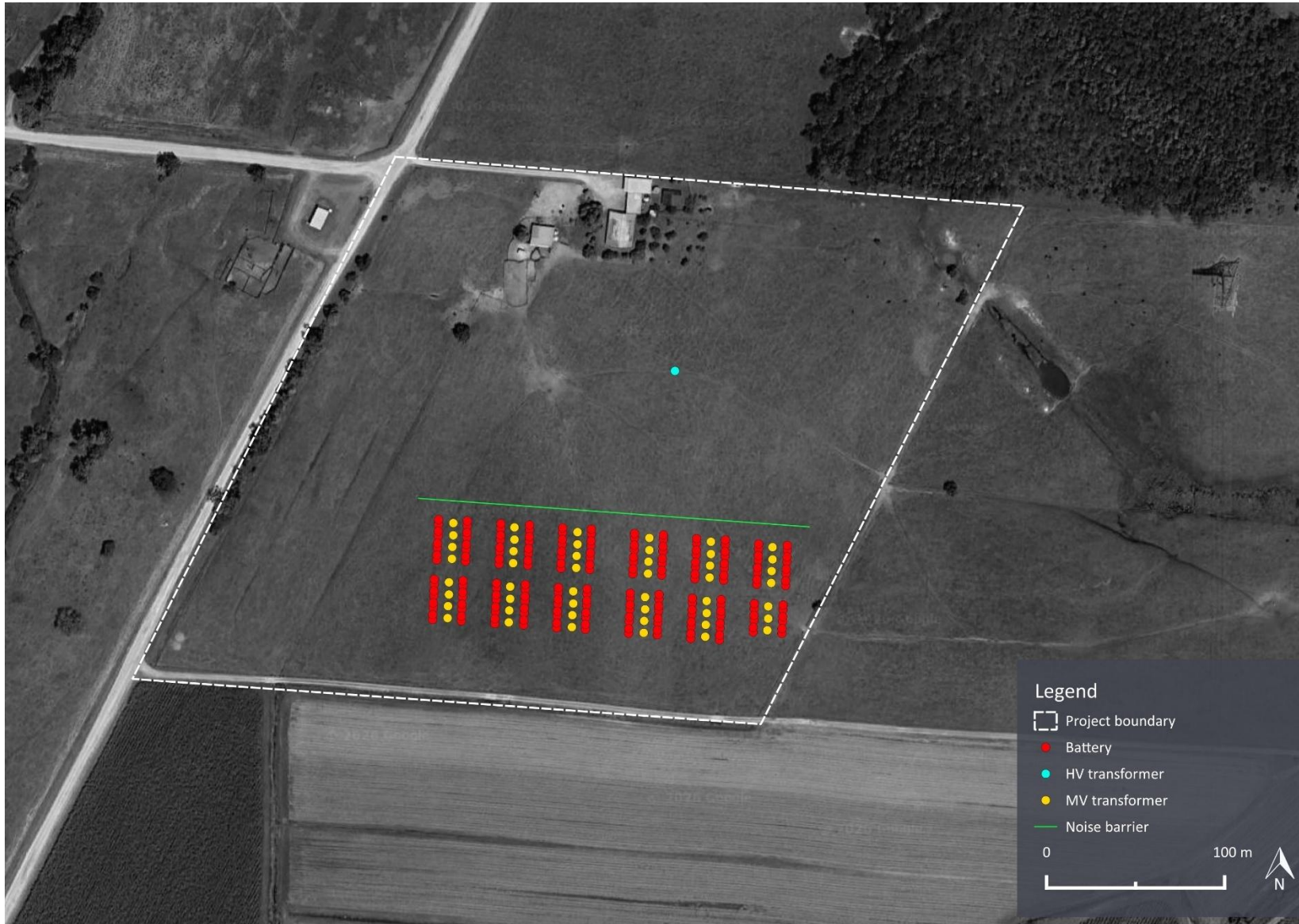
Figure 2: Project layout and indicative noise source locations
