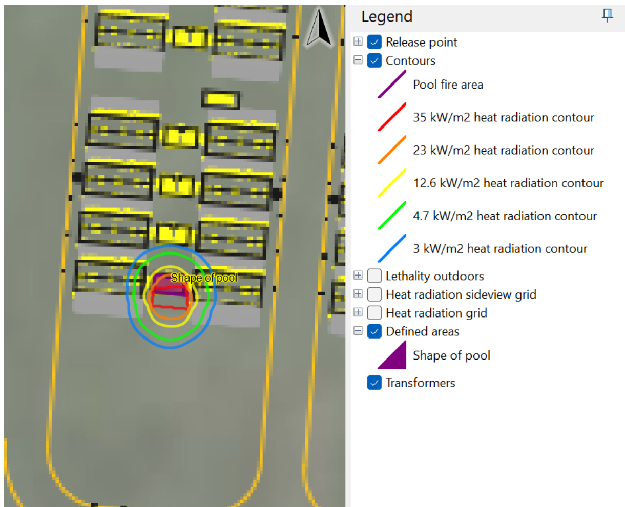
Figure 5-2: MV Transformer Fire Radiant Heat Contours
