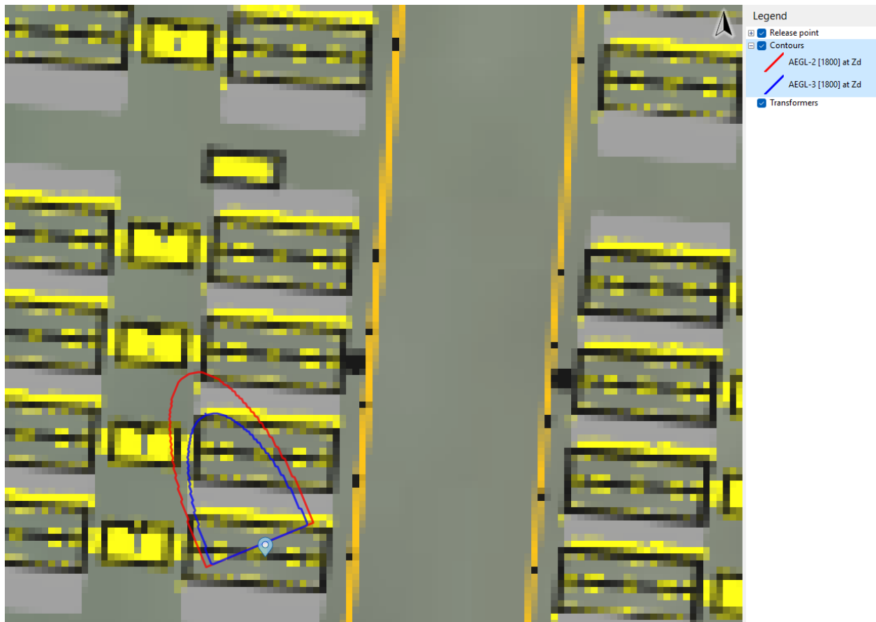
Figure 5-4: HF AEGL 5 Minute Exposure Contours Proximity to Offsite Receptors.
