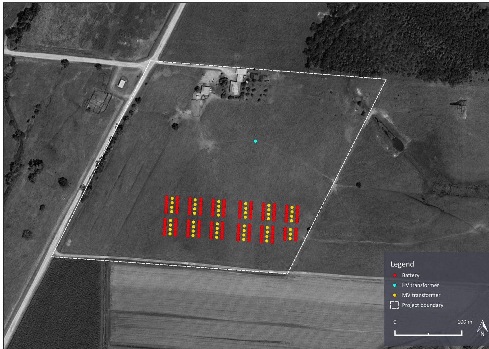
Figure 2: Project layout and indicative noise source locations
