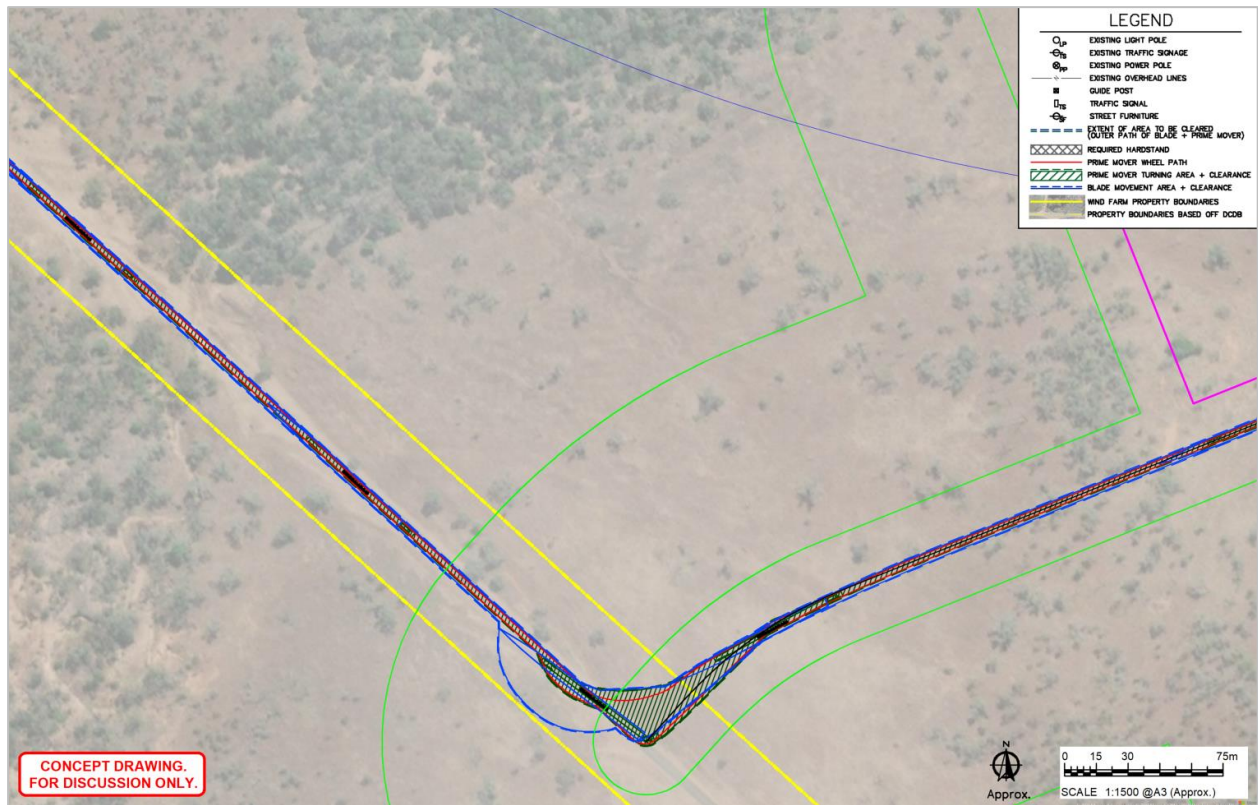
Figure 5.8 Project Area Access #2 Swept Path of Wind Turbine Blade Transport Accessing Project Site
