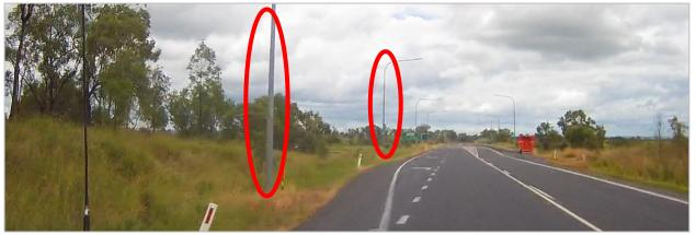
Figure 3.43 Street view of reviewed intersection facing west and light poles to be removed
