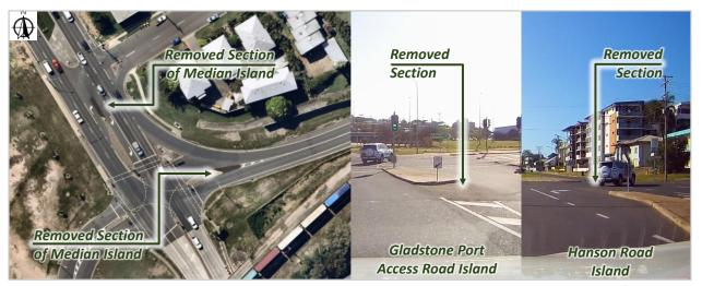
Figure 2.4 Median Island sections removed from intersection of Gladstone Port Access Road / Hanson Road.
