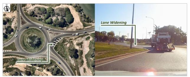
Figure 2.5 Lane widening on eastern approach to Hanson Road / Blain Drive / Alf O'Rourke Drive roundabout.
