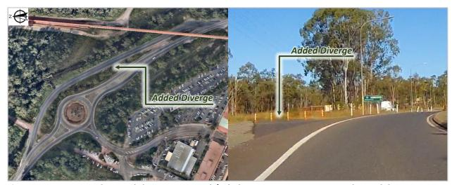
Figure 2.7 Bypass road around the Hanson Road / Gladstone Mount Larcom Road roundabout.
