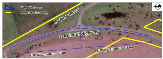
Figure 7.3 Safe Intersection Sight Distance – Leichardt Highway / Defence Road intersection
