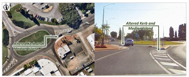
Figure 2.9 Kerb and median island alterations on eastern approach to Lord Street / Bryan Jordan Drive roundabout.
