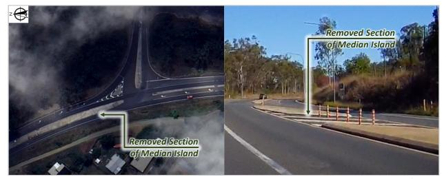
Figure 2.8 Median Island sections removed from intersection of Gladstone Mount Larcom Road / Bruce Highway.
