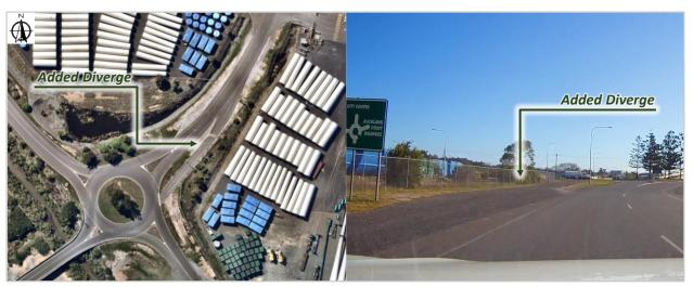
Figure 2.3 Diverge pavement added for movements through Mark Fenton Drive / Gladstone Port Access Road Roundabout.
