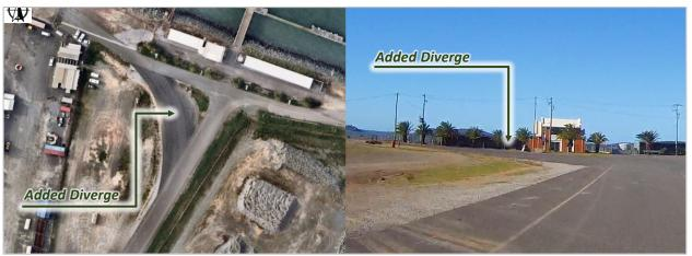
Figure 2.2 Diverge lane provided to intersection of Macfarlane Road / Mark Fenton Drive.
