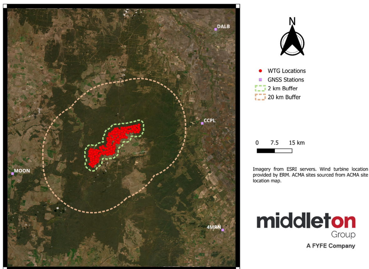
Figure 10: GNSS Station locations relative to WTG layout
